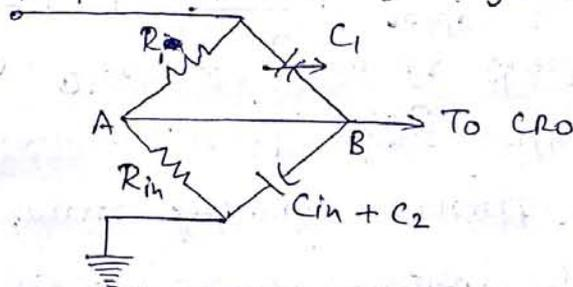
The compensating capacitor is adjusted so as to get balanced bridge condition.
