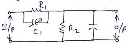
If the time constant  $R_1 C_1$  of the probe is equal to  $R_2 C_2$  of the CRO, the complex waveform will be passed through the probe without distortion.
