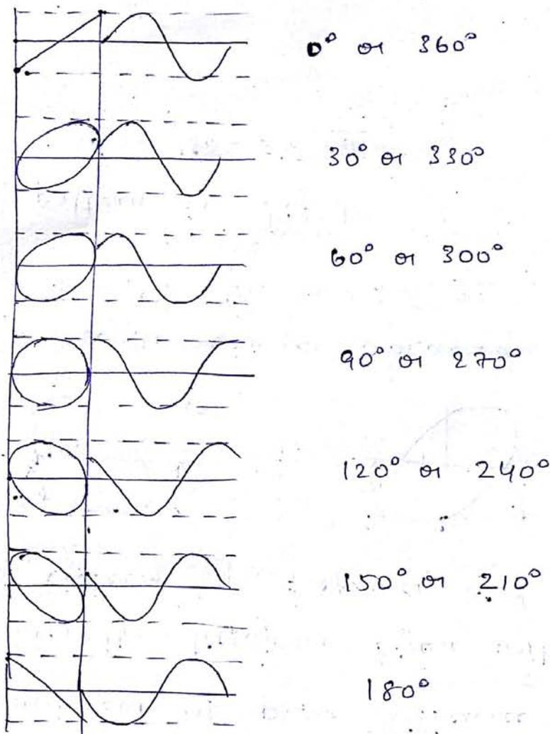
problem :- the Lissajous figure is obtained on the CRO as shown. Find the phase difference between the two waves applied.
