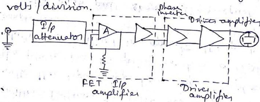
The vertical amplifier is kept within its signal handling capability by proper selection of the I/p attenuator switch.
