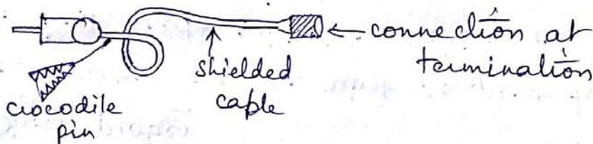
The shunt capacitance effect of such probe at high freq can be reduced by placing a carbon resistor in series with the test leads.
