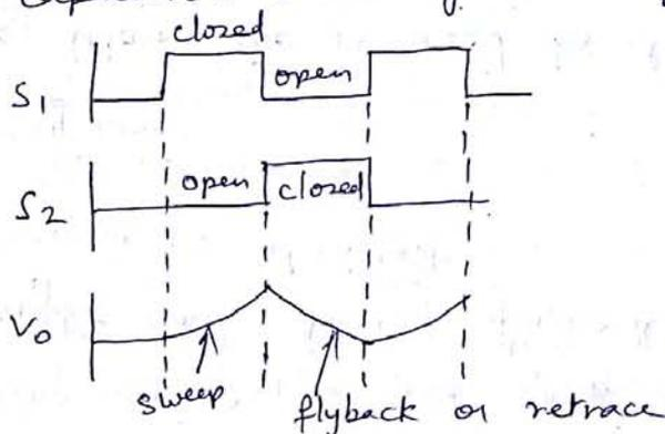
During sweep time the spot moves from left to right and during flyback or retrace time, the screen is blanked.
