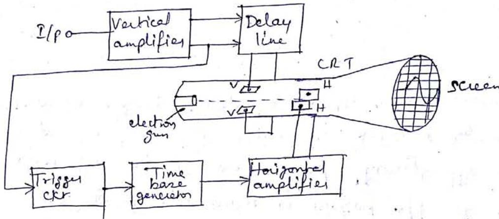
CRT - The cathode ray tube is the heart of the CRO, used to emit the electrons required to strike the phosphor screen to produce the spot for display
