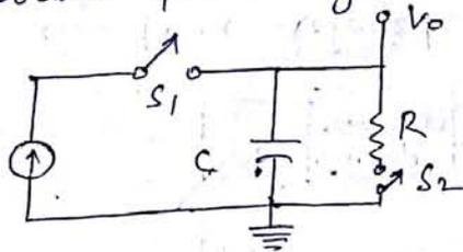
When switch  $S_1$  is closed,  $S_2$  is open, capacitor charges to produce linear ramp. The sweep rate can be controlled by changing the value of capacitor or charging current. When capacitor is charged upto the maximum current,  $S_2$  is closed and  $S_1$  open. The capacitor discharges through resistor  $R$ .
