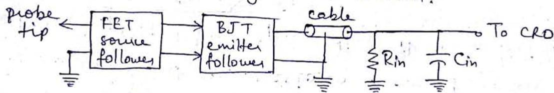
FET is used as an active element to amplify the signal. The voltage gain of FET source follower is unity but it provides a power gain due to which the input impedance increases.
