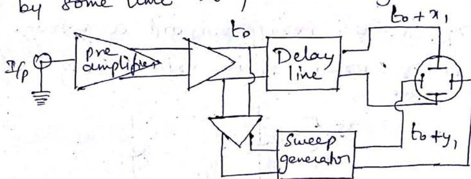
As the signal is delayed, the sweep generator output gets enough time to reach the horizontal plates before reaching the vertical plates. If the trigger pulse is picked off at a time  $t = t_0$ , after passing through the main amplifier, the signal is delayed by  $x_1$  nano seconds.
