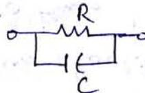
A coaxial cable connects probe head to CRO input. Let  $C_2$  be the probe cable equivalent capacitance. Input resistance and capacitance of CRO can be referred as  $R_{in}$  and  $C_{in}$ .
