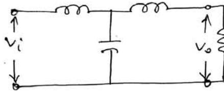
The T-section acts as a low pass filter having cut off frequency as
