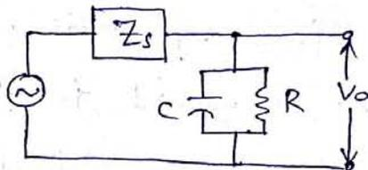
The resistance and capacitance of a CRO is high, hence a shielded cable is necessary. If shielded cables are not used, the stray fields produce interference on the pattern on the CRO. The shielded cable provides high input impedance with a low capacitance.
