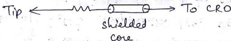
Such a probe is called isolation probe.
