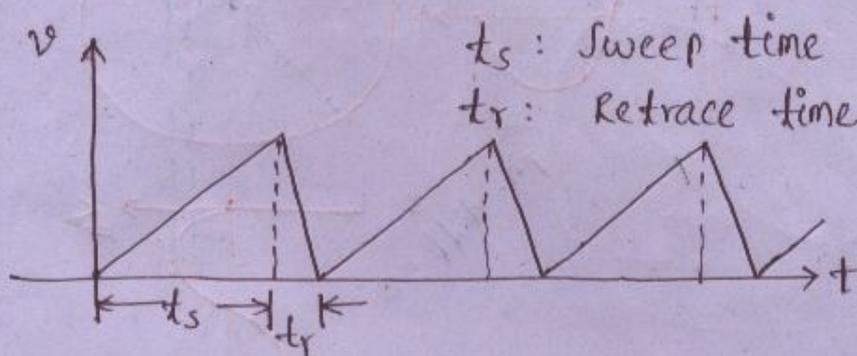
During sweep time, beam moves from left to right most pos. on the screen.
