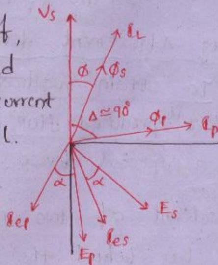
\* current through shunt coil  $I_p$  lagging  $V$  by  $\Delta$  nearly  $= 90^\circ$  ( $\Delta \approx 90^\circ$ ).
