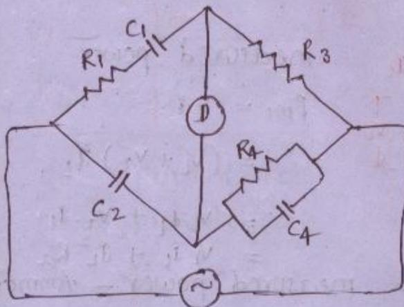
$$C_1 = \frac{R_4}{R_3} \times C_2$$
