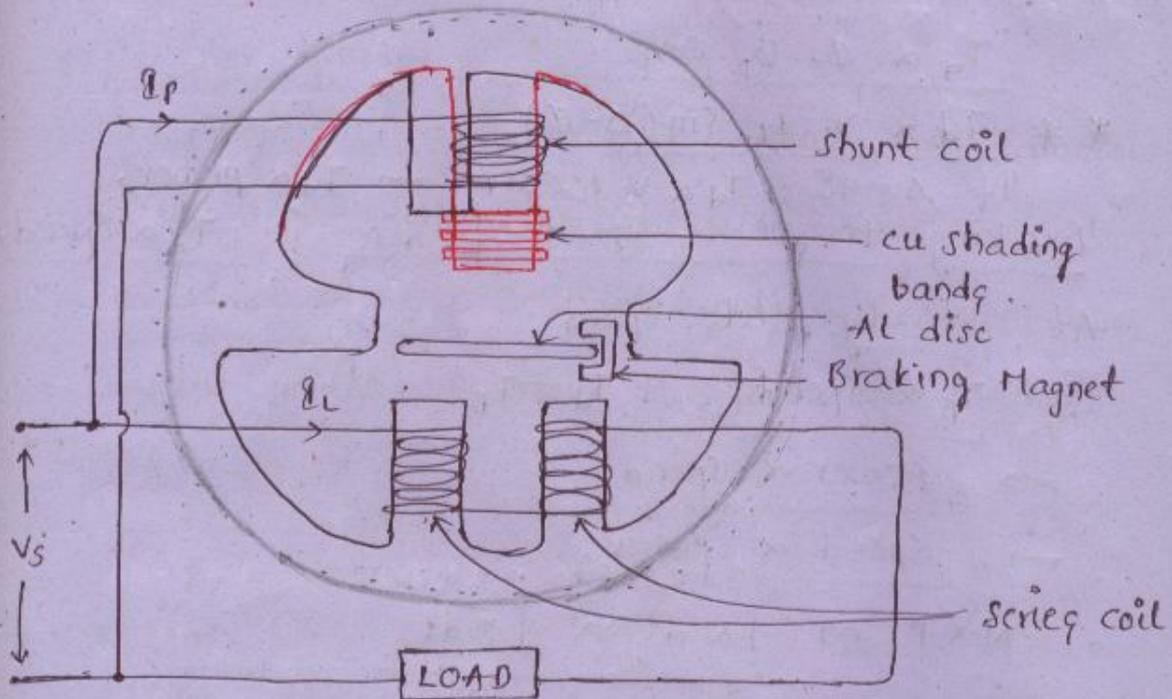
Energy meter consists of, coil in series with load and carries the load current is known as series coil.
