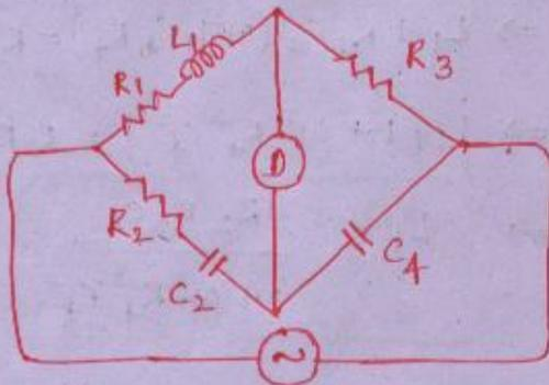
This is only <sup>inductance</sup> bridge which consists of two capacitances.
