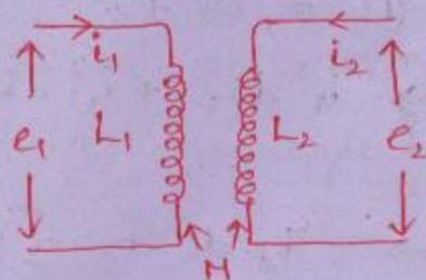
Operating principle is based on change in M b/w the two coils.
