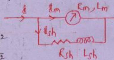
$$= \frac{R_{sh} \sqrt{1 + \left(\frac{\omega L_{sh}}{R_{sh}}\right)^2}}{R_m \sqrt{1 + \left(\frac{\omega L_m}{R_m}\right)^2}}$$
