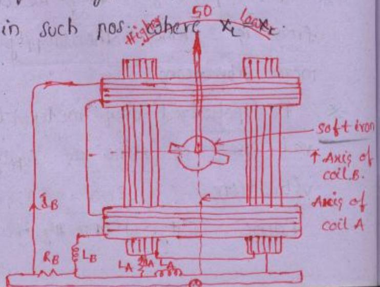
The meter consists of 2 coils mounted  $\perp^{\text{er}}$  to each other. Each coil is divided into 2 parts. coil A is connected in series with resistance  $R_A$  and whole setup placed across  $L_A$ .
