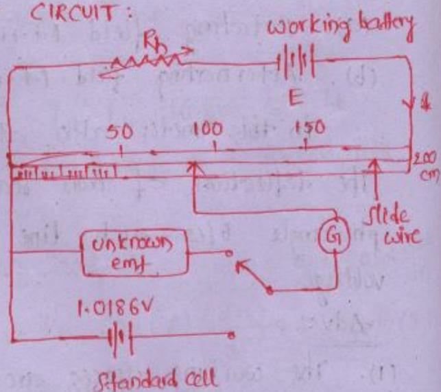
potentiometer is required to be standardized before making measurement by a std. cell.
