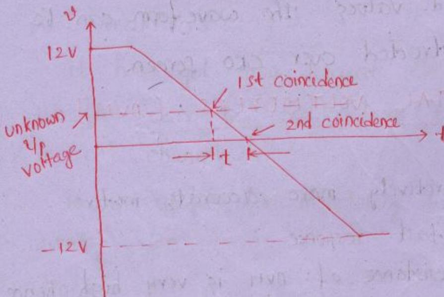
Operating principle is to measure the time that a linear ramp takes time to change from unknown  $\pm 1\%$  volt. level to ground
