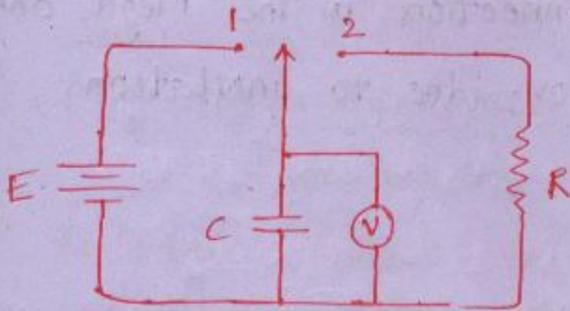
capacitor gets charge towards supply voltage by connecting to pos. 1.
