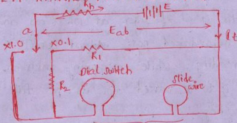
This P.M is useful to select two ranges without disturbing the calculations.
