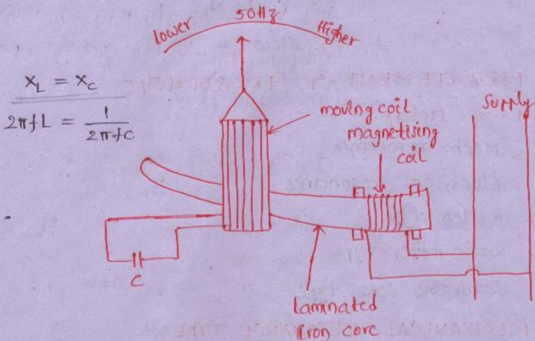
Operating principle based on electrical resonance.
