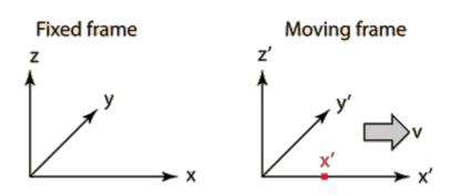
The primed frame moves with velocity v in the x direction with respect to the fixed reference frame. The reference frames coincide at t=t'=0. The point x' is moving with the primed frame.
