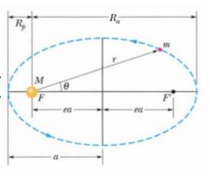
ellipse's center, with e being the eccentricity of the ellipse The semimajor axis a of. the ellipse, the perihelion (nearest the Sun) distance  $R_p$ , and the aphelion (farthest from the Sun) distance  $R_a$  are also shown.
