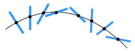
Fig(6) The center of mass of a thrown rigid rod follows a parabolic trajectory while the rod rotates about the center of mass.
