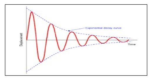
FIGURE: Displacement-time graph for the damped harmonic oscillations
