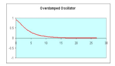
Such a motion is called the dead beat or a periodic motion. This type of motion is used in the dead beat galvanometer.
