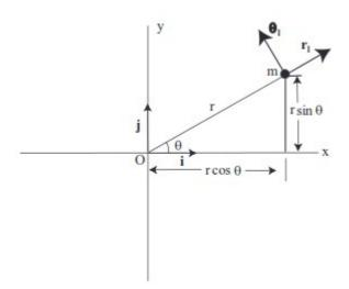
Fig(1):Polar coordinate system of a particle moving in the xy plane. Since the vectorial nature of the central force is expressed in terms of a radial vector from the origin it is most natural (though not required!) to write the equations of motion in polar coordinates. In earlier lectures we derived the expression for the acceleration of a particle in polar coordinates
