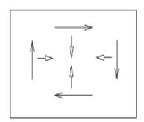
drawn various particle velocities, together with the Coriolis force experienced by the particle. We see that the effect of the Coriolis force is that a free particle travelling on the plane will move in a clockwise direction.
