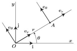
Since we are dealing with free vectors, we can translate the polar reference frame for a given point  $(r, \theta)$ , to the origin, and apply a standard change of basis procedure. This will give, for a generic vector A,
