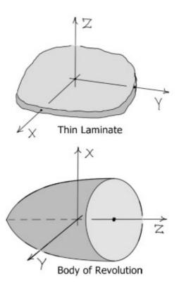
Products of inertia are found either by measurement or by calculation. Calculations arebased on direct integrationor on the "body build-up" technique. In the body build-up technique, products of inertia of simple shapes are added to estimate the products of inertia of a composite shape. The products of inertia of simple shapes (about their individual mass centers) are found in standard inertia tables. These values are transferred to axes through the composite mass center using the
