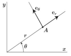
The position vector of a particle has a magnitude equal to the radial distance, and a direction determined by  $e_r$ . Thus,
