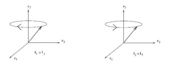
**Fig:** The precession of the spin: the direction of precession depends on whether the object is short and fat  $(I_3 > I_1)$  or tall and skinny  $(I_3 < I_1)$
